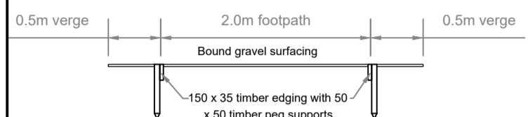
SECTION 1 2.0m leisure footpath (1:50@A1)
